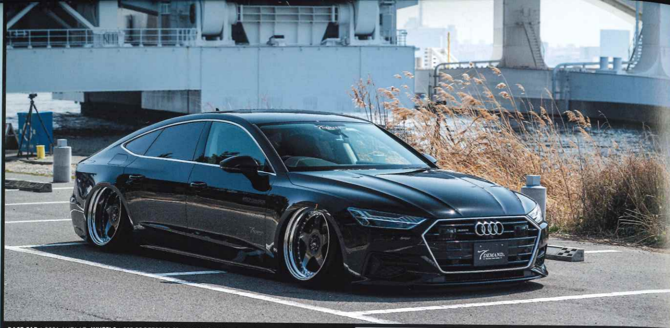
BASE CAR : 2021 AUDI A7 WHEELS : SSR PROFESSOR SP6 UNDER (F=20x10.5J-3 / R=20x10.5J-8) TIRES : NITTO INVOI(F&R=245/30-20) SUSPENSIONS : T-DEMAND (AIR-SUS SRIM3BAG / HARD LINE BUTTERFLYα V8 SYSTEM) T-DEMANDPROARM (FRONT UPPER-ARM / FRONT LOWERARM / TENSIONARM / TIERODEND / REAR UPPERARM / TOECONTROLARM / REAR TENSIONARM / SHORTKNUCKLE) BRAKE : T-DEMAND BRAKE SYSTEM
